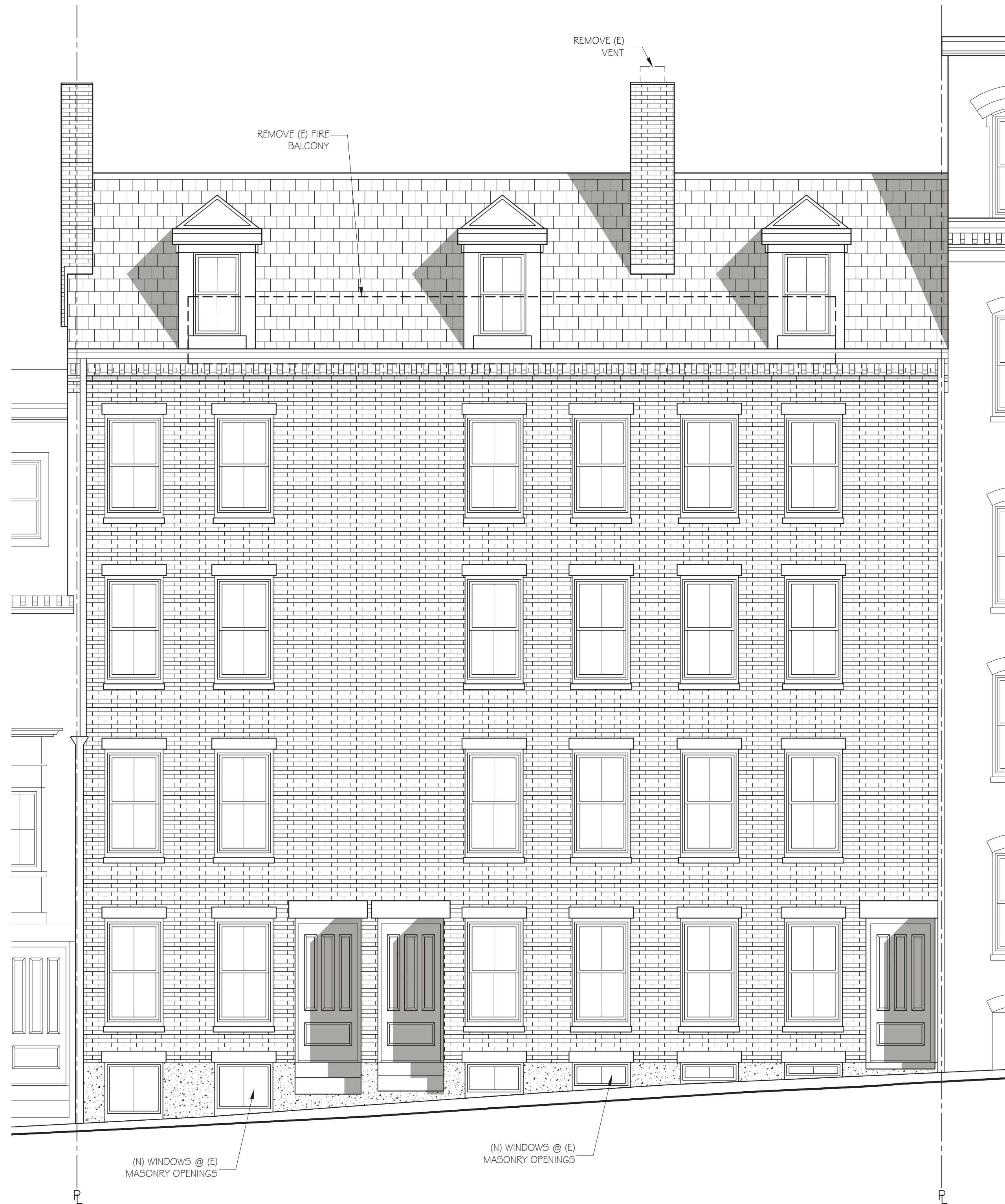
EAST BUILDING ELEVATION \frac{1}{4}'' = 1'-0''
