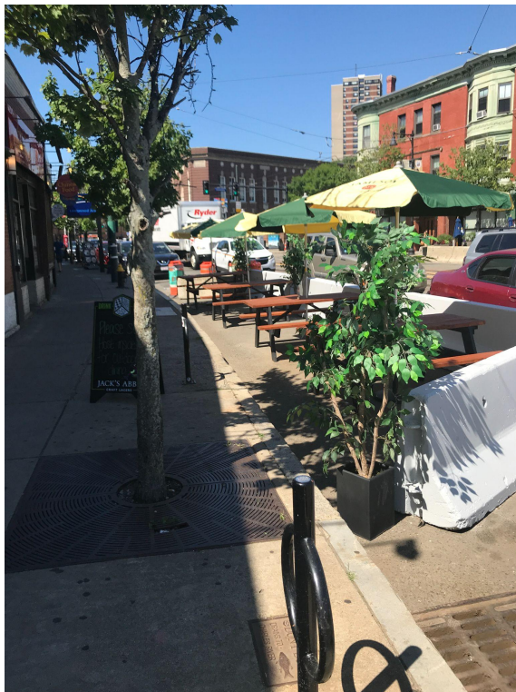
Water-filled jersey barriers To be filled with water by Licensee
